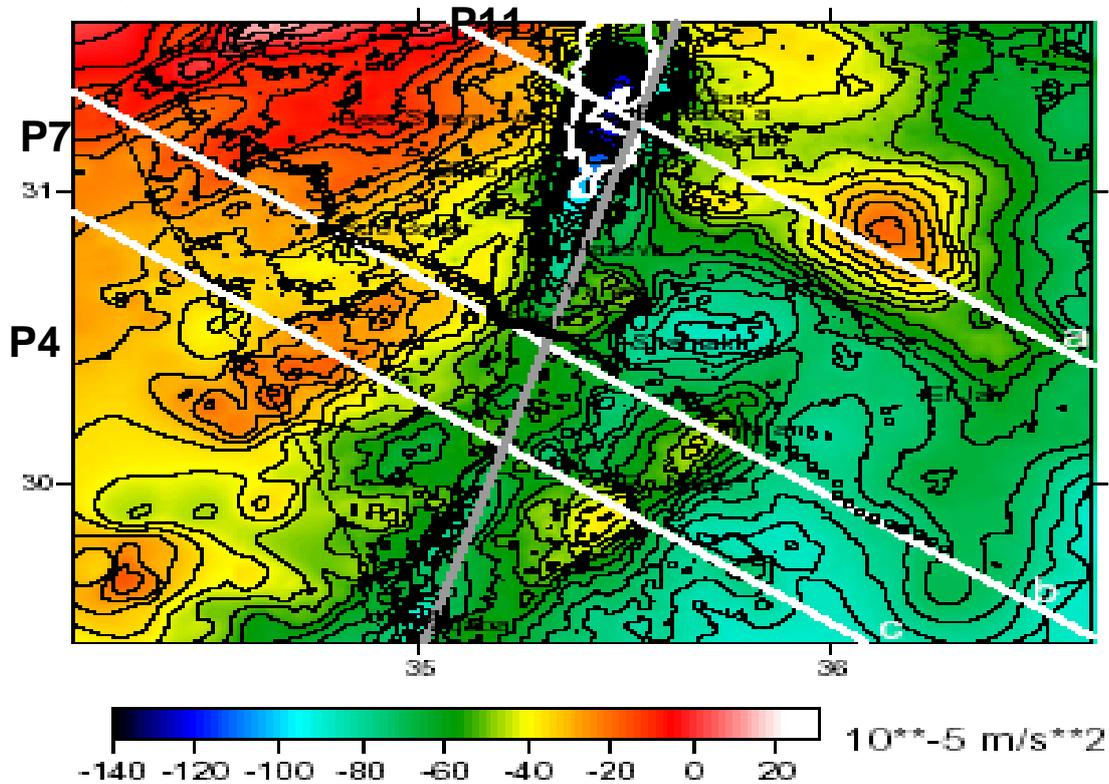
**Figure 3.** Compiled Bouguer anomaly map of the southern part of the Jordan Dead Sea Transform (contour interval 5 mGal). The solid lines a, b, c (white) show the locations of the 3-dimensional modelling vertical planes p4, p7, p11 among 14 modelled cross-section.
