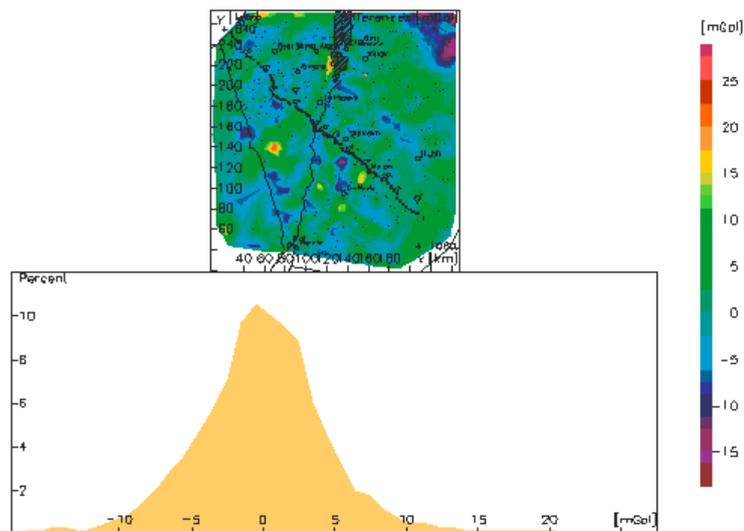
**Fig** *Histogram of gravity differences between measured and computed Bouguer anomalies (correlation coefficient 0.98). Also shown is the misfit between the measured and computed Bouguer anomaly map of the study area (contour interval 1 mGal).*
