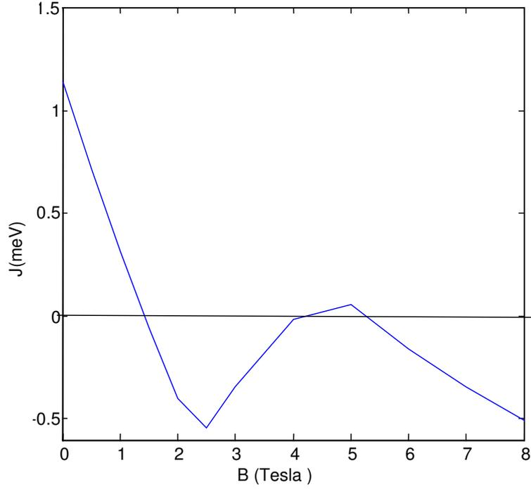
**Figure 2.** The triplet-singlet energy splitting ( $J$  in meV) for two electron quantum dot against the magnetic field ( $B$  in Tesla) for confinement strength  $\hbar\omega_0 = 3$  meV. [Material parameters for GaAs are:  $m^* = 0.067 m_e$ ,  $\kappa = 12.4$ ,  $R^* = 5.93$  meV,  $a^* = 9.8$  nm,  $g^* = -0.44$ ].
