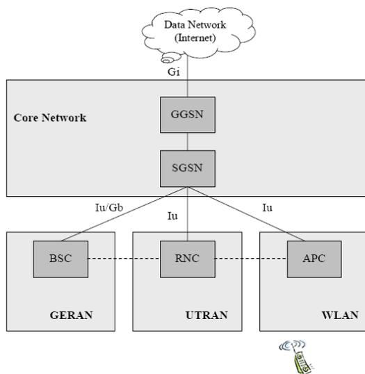
Fig. 3: WLAN/3GPP architecture
