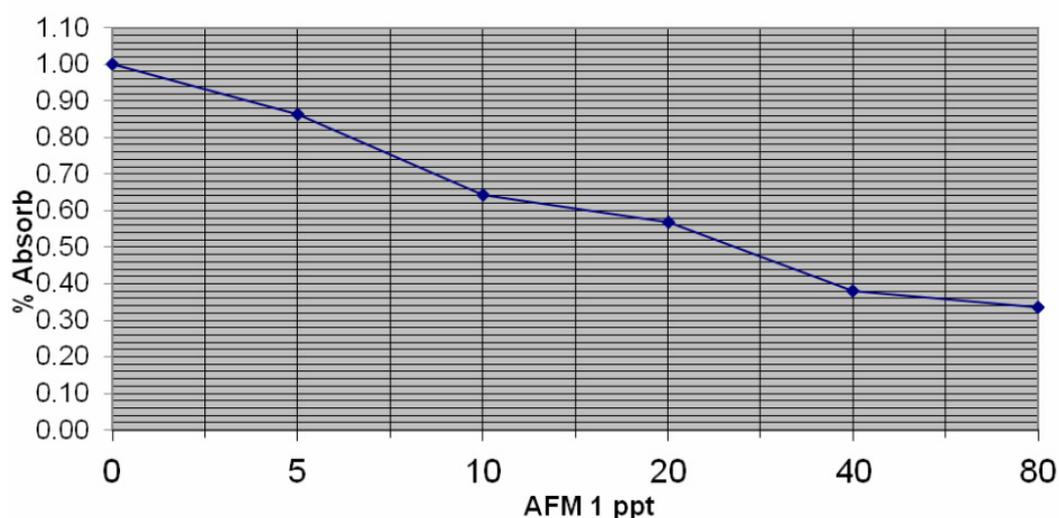
**Figure 1** Calibration curve of aflatoxin M1 standards 0 ppt (zero standard), 5 ppt, 10 ppt, 20 ppt, 40 ppt, and 80 ppt. The optical density (O.D.) of each standard based on the zero standard.
