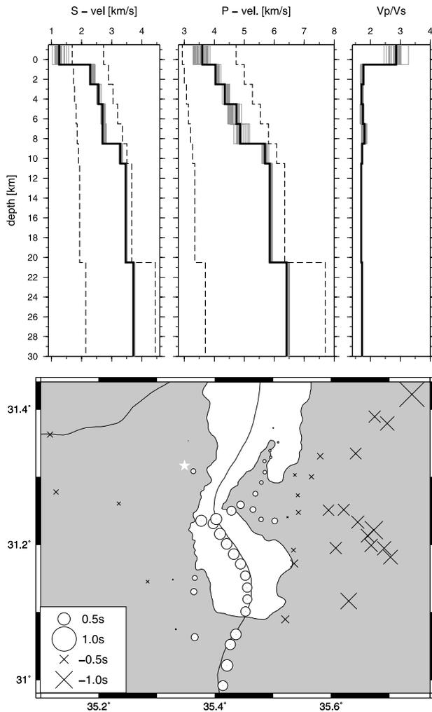
**Figure 2.** (Top panel) 1-D velocity models for *S* and *P* waves and  $v_p/v_s$  ratio. All resulting models from 36 different starting models are shown in grey. Solid black lines indicate the best final model with lowest rms. Dashed lines indicate the limits of the used starting models. (Bottom panel) Corresponding *P*-wave station corrections. The reference station is indicated by a star.
