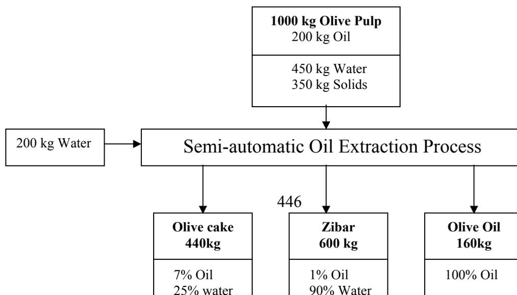
Figure 1: Mass Balance – Semi-automatic oil extraction process
