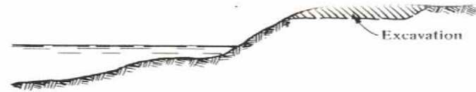
(a) Excavation at top of slope
