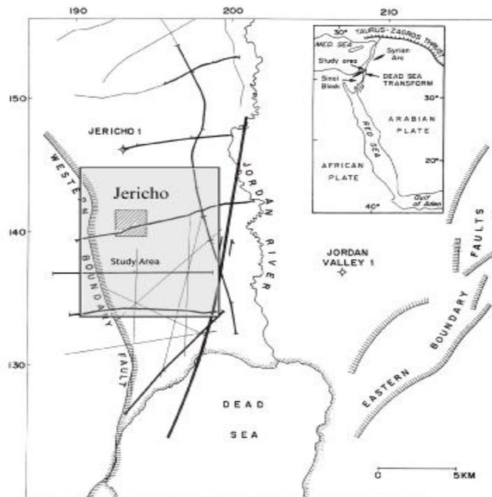
**Figure 1:** Location map of present study, showing the location of the study area, the seismic reflection lines [20] and the deep wells in the area. The thick line marks the location of the plate transform [19].
