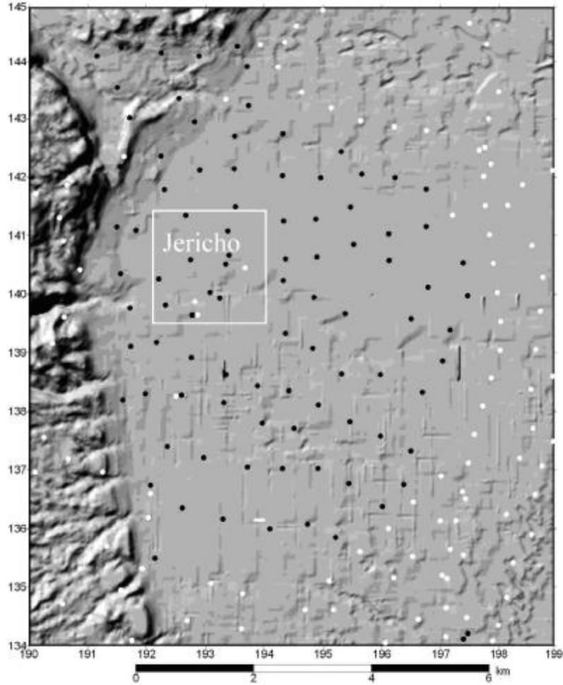
**Figure 3:** Gravity coverage map of the Jericho area; black dots donate the new gravity stations; white dots are the old stations.
