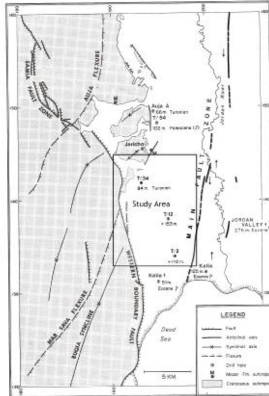
**Figure 2:** Simplified geological map of the study area. Also shown are wells in which pre-rift Upper Mesozoic and Tertiary sediments were found; numbers indicate depth to pre-rift sediments, and their ages appear when known. The transform is recognized by the terrace (bold dashed lines) which it forms in the white chalk of the Pleistocene Lisan Formation; it is marked by arrows.
