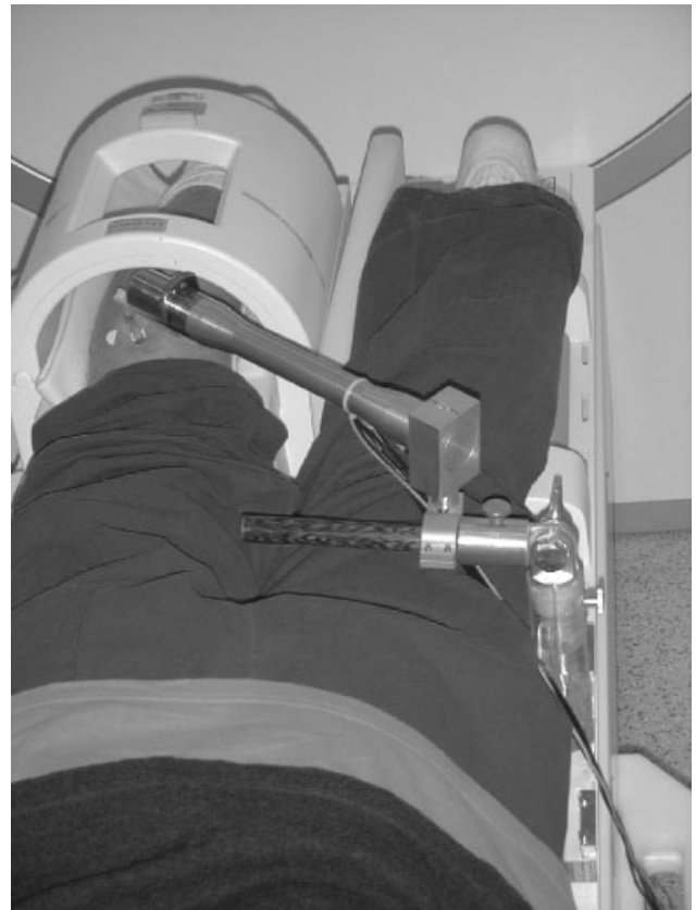
Figure 3. Setup using a transmit–receive extremity coil for examination of the calf muscles, i.e. the gastrocnemius and the soleus. Apart from RF coil used and positioning of the actuator, the same principle setup was used for examination of the biceps and the forearm
