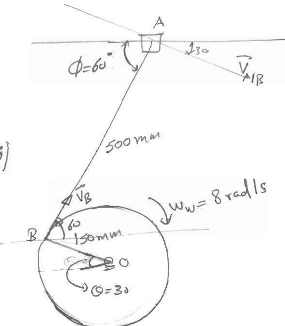
$$\Rightarrow \frac{V_A}{\sin \theta} = \frac{V_B}{\sin 30^\circ} \Rightarrow V_A = \frac{V_B}{\sin 30^\circ} = \frac{1.2}{\sin 30^\circ} = 2.4 \text{ m/s} \rightarrow$$
