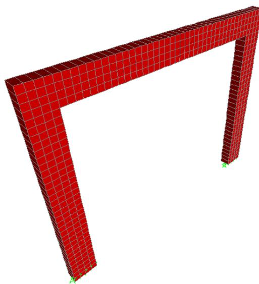
**Figure 2:** Finite element model for portal frame in 3-D
