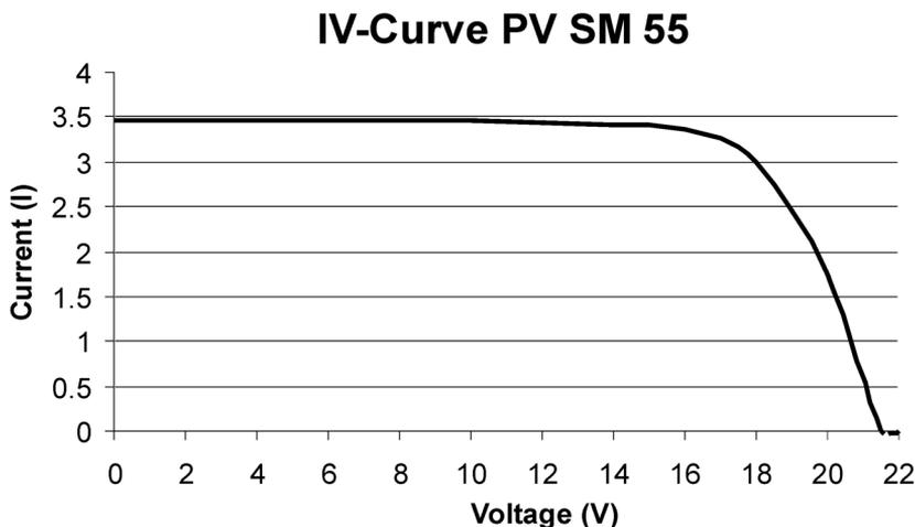
FIGURE 2 IV-curve for PV-module (Type SM55).
