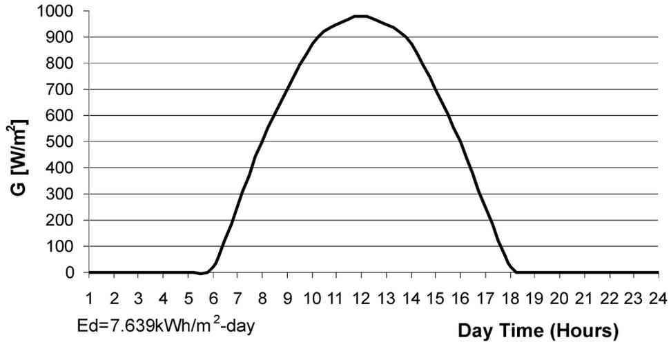
FIGURE 4 Solar radiation intensity according to SSD-model.
