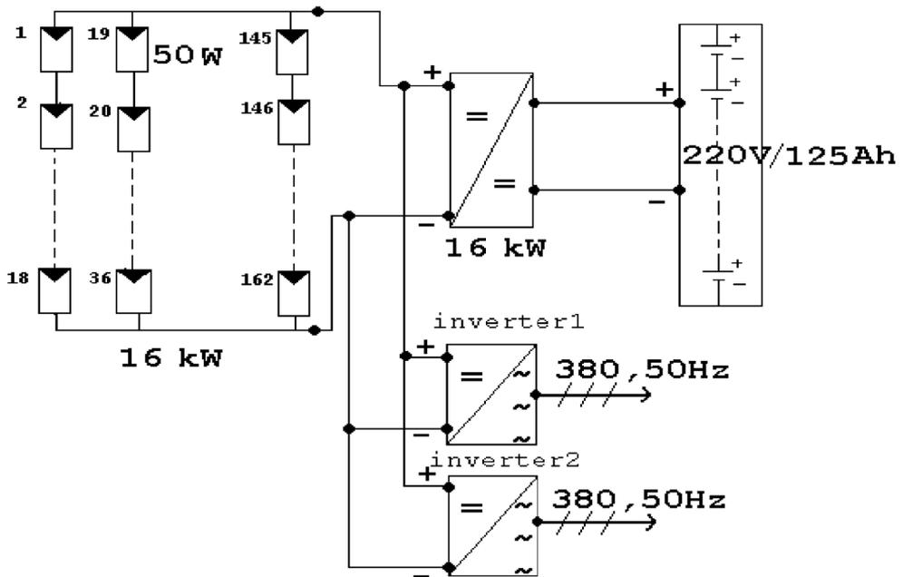
FIGURE 3 The interconnection of the PV generator (Slope  $32^\circ$ , Azimuth =  $0^\circ$ ).
