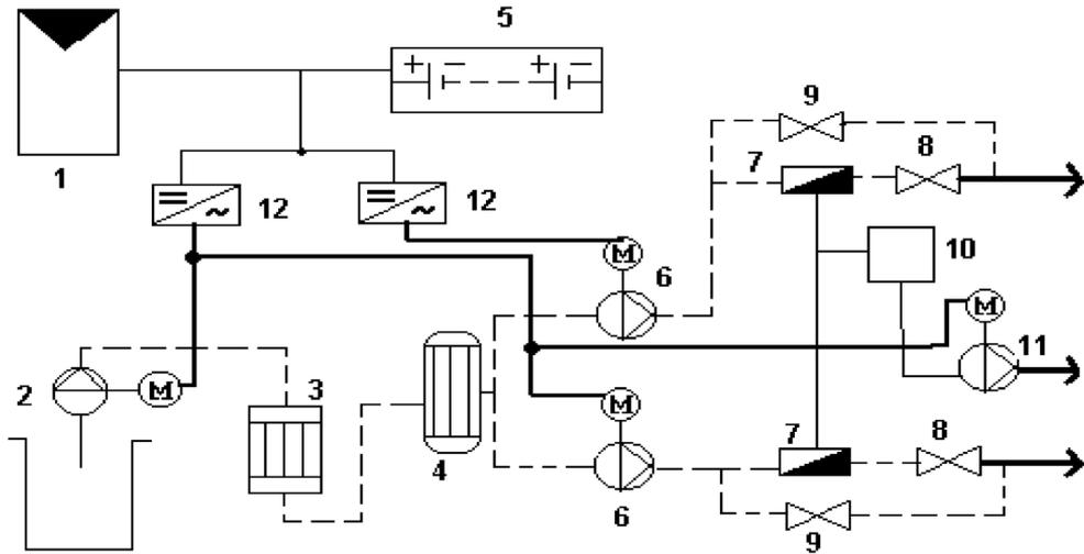
FIGURE 1 Block diagram of the proposed PV-powered RO desalination plant for brackish water in Al Maleh village. 1, Solar Generator; 2, Well Pump; 3, Sand Filter; 4, Cartridge Filter; 5, Battery Block; 6, High Pressure Pumps; 7, RO-Modules; 8, Regulating Valves; 9, Starting Valves; 10, Product Water Storage; 11, Product Water Pump; 12, DC/AC 3 Phase Inverter.
