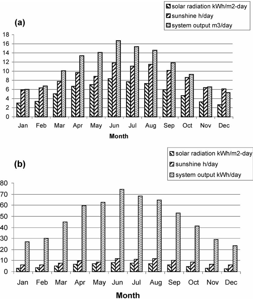
FIGURE 6 Simulation results of the PV-powered brackish water desalination system in Al Maleh village.
