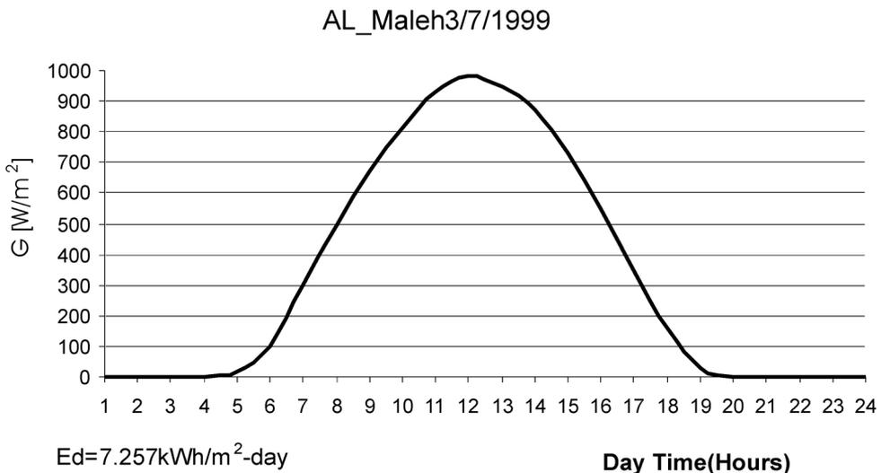
FIGURE 5 The solar radiation measurement in Al Maleh village area.
