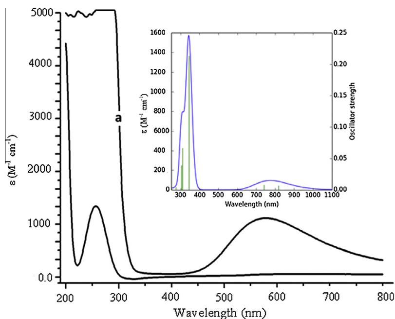
**Fig. 2.** UV-Vis spectrum of **2** in water, Inset shows simulated absorption spectrum, (green line) based on TD-DFT calculations, compared to excitation energies and oscillator strengths. (For interpretation of the references to color in this figure legend, the reader is referred to the web version of this article.)
