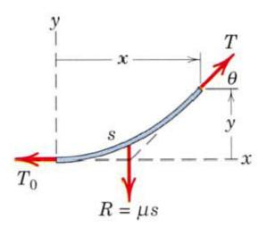
$$T^{2} = T_{H}^{2} \left( 1 + \sinh^{2} \frac{\mu x}{T_{H}} \right) = T_{H}^{2} \cosh^{2} \frac{\mu x}{T_{H}}$$
