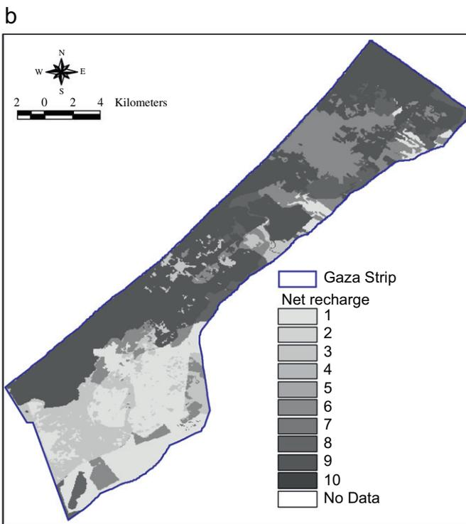
Fig. 5. The rated maps of (a) depth to water and (b) net recharge. The rating score 1 implies a minimum impact on vulnerability while the score 10 indicates the maximum impact.
